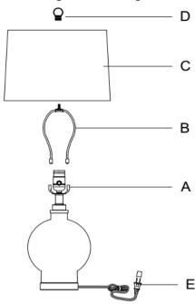
**Step 3:** Finally, connect the plug of lamp (E) to a GFCI outlet.
