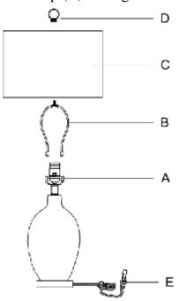
**Step 3:** Finally, connect the plug of lamp (E) to a GFCI outlet.
