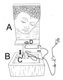
**Step 2:** Fill the basin (B) with clean water, making sure the pump (C) is fully submerged. **Note:** The maximum water level should be approximately 1.0 inches below the top edge of the basin (B).
