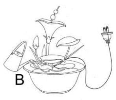
**Step 3:** Finally, connect the plug of pump (C) to a GFCI outlet. **WARNING:** Always disconnect the pump (C) before placing your hands in the water.
