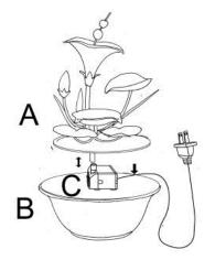
**Step 2:** Fill the basin (B) with clean water, making sure the pump (C) is fully submerged. **Note:** The maximum water level should be approximately 1.0 inches below the top edge of the basin (B).
