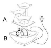
**Step 2:** Fill the basin (B) with clean water, making sure the pump (C) is fully submerged. **Note:** The maximum water level should be approximately 1.0 inches below the top edge of the basin (B).
