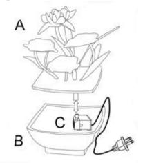
**Step 3:** Fill the plastic basin (B) with clean water, making sure the pump (C) is fully submerged.
