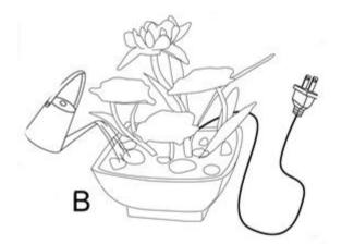
**Step 4:** Finally, connect the plug of pump (C) to a GFCI outlet. **WARNING:** Always disconnect the pump (C) before placing your hands in the water.
