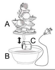
**Step 2:** Fill the basin (B) with clean water, making sure the pump (C) is fully submerged. **Note:** The maximum water level should be approximately 1.2 inches below the top edge of the basin (B).
