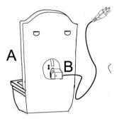
**Step 2:** Fill the bottom basin (A) with clean water, making sure the pump (B) is fully submerged.
