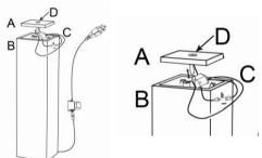
**Step 2:** Fill the basin (B) with clean water, making sure the pump (C) is fully submerged. **Note:** The maximum water level should be approximately 1.2 inches below the top edge of the basin (B).
