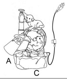
**Step 3:** Finally, connect the plug of pump (C) to a GFCI outlet.
