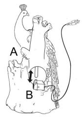
**Step 2:** Fill the basin (A) with clean water, making sure the pump (B) is fully submerged. **Note:** The maximum water level should be approximately 1.2 inches below the top edge of the basin (A).
