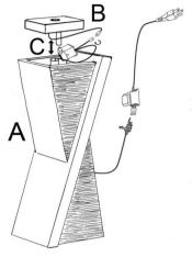
**Step 2:** Fill the product (A) with clean water, making sure the pump (C) is fully submerged.
