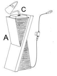
**Step 3:** Finally, connect the plug of pump (C) to a GFCI outlet.
