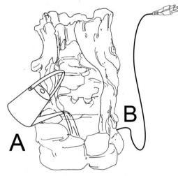
**Step 3:** Finally, connect the plug of pump (B) to a GFCI outlet. **WARNING:** Always disconnect the pump (B) before placing your hands in the water.
