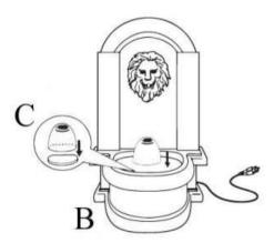
**Step 3:** Fill base (B) with clean water. Note: The maximum water level should be no higher than the water-level line on platform (C).
