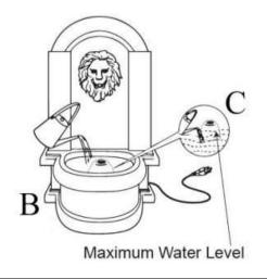
**Step 4:** Finally, connect plug of pump (D) to a GFCI outlet.
