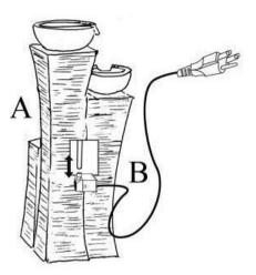
**Step 2:** Fill the basin (A) with clean water, making sure the pump (B) is fully submerged. **Note:** The maximum water level should be approximately 1.2 inches below the top edge of the basin (A).
