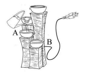
Step 3: Finally, connect the plug of pump (B) to a GFCI outlet.WARNING: Always disconnect the pump (B) before placing your hands in the water.
