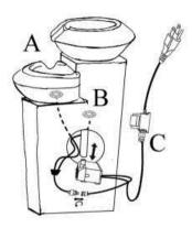
**Step 2:** Fill the product (A) with clean water, making sure the pump (C) is fully submerged.
