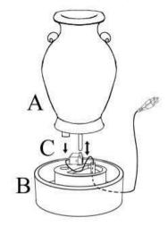
**Step 2:** Fill the basin (B) with clean water, making sure the pump (C) is fully submerged. **Note:** The maximum water level should be approximately 1.2 inches below the top edge of the basin (B).
