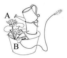
**Step 2:** Fill the basin (A) with clean water, making sure the pump (B) is fully submerged. **Note:** The maximum water level should be approximately 1.2 inches below the top edge of the basin (A).
