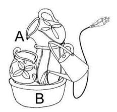
**Step 3:** Finally, connect the plug of pump (B) to a GFCI outlet.
