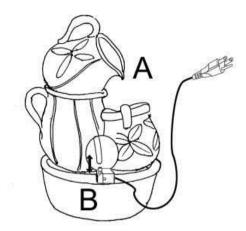
**Step 2:** Fill the basin (A) with clean water, making sure the pump (B) is fully submerged. **Note:** The maximum water level should be approximately 1.2 inches below the top edge of the basin (A).
