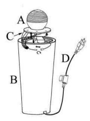
**Step 2:** Fill the base (B) with clean water, making sure the pump (D) is fully submerged **Note:** The maximum water level should be approximately 1.2 inches below the top edge of the basin (B).
