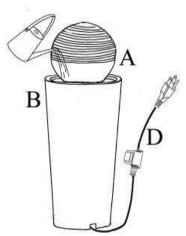
$\textbf{Step 3:} \ \, \textbf{Finally, connect the plug of pump (D) to a GFCI outlet}.$
