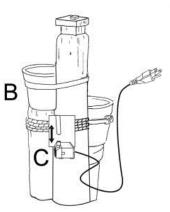
**Step 2:** Align the top solar post light (A) to pot pillar (B).
