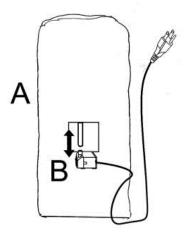
**Step 2:** Fill the basin (A) with clean water, making sure the pump (B) is fully submerged. **Note:** The maximum water level should be approximately 1.2 inches below the top edge of the basin (A).
