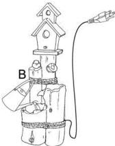
**Step 3:** Finally, connect the plug of pump (B) to a GFCI outlet.
