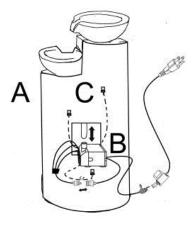
**Step 2:** Fill the basin (B) with clean water, making sure the pump (B) is fully submerged. **Note:** The maximum water level should be approximately 1.2 inches below the top edge of the basin (A).
