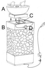
**Step 2:** Fill the product (A) with clean water, make sure the pump (C) is fully submerged. **Note:** The maximum water level should be approximately 1.2 inches below the top edge of the basin (A).
