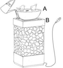
**Step 3:** Finally, connect the plug of pump (C) to a GFCI outlet. **WARNING:** Always disconnect the pump (C) before placing your hands in the water.
