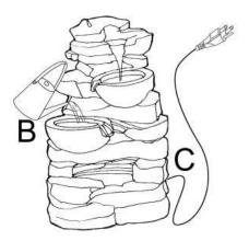
**Step 4:** Finally, connect the plug of pump (C) to a GFCI outlet.
