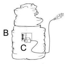
**Step 3:** Fill the basin (B) with clean water, making sure the pump (C) is fully submerged. **Note:** The maximum water level should be approximately 1.2 inches below the top edge of the basin (B).
