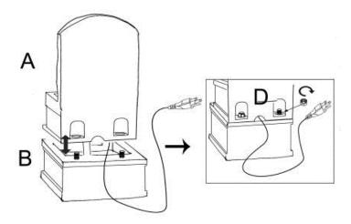
**Step 3:** Fill the basin (B) with clean water, making sure the pump (C) is fully submerged. **Note:** The maximum water level should be approximately 1.2 inches below the top edge of the basin (B).
