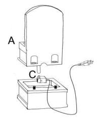
**Step 2:** Align and attach the top part (A) to the bottom (B), using the bolts and washers to fix both parts.
