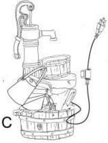
Step 5: Finally, connect the plug of pump (D) to a GFCI outlet.WARNING: Always disconnect the pump (D) before placing your hands in the water.
