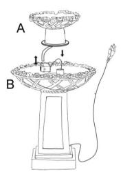
**Step 4:** Fill the basin (B) with clean water, making sure the pump (D) is fully submerged.
