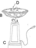
**Step 3:** Connect the water hose to the pump, then carefully attach the first basin (A) to the Large Basin (B), making sure to place the pump in the center of the Large Basin (B).
