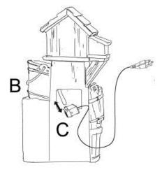
**Step 3:** Fill the basin (B) with clean water, making sure the pump (C) is fully submerged. **Note:** The maximum water level should be approximately 1.2 inches below the top edge of the basin (B).
