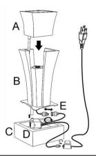
**Step 3:** Fill the bottom basin (C) with clean water, making sure the pump (D) is fully submerged.
