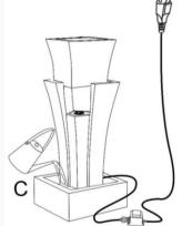
**Step 4:** Finally, connect the plug of pump (D) to a GFCI outlet. **WARNING:** Always disconnect the pump (D) before placing your hands in the water.
