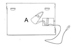
**Step 3:** Finally, connect the plug of pump (B)to a GFCI outlet.
