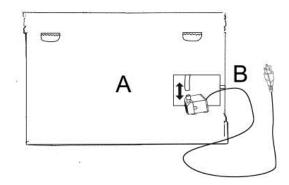
**Step 2:** Fill the basin (A) with clean water, making sure the pump (B) is fully submerged. **Note:** The maximum water level should be approximately 1.2 inches below the top edge of the basin (A).
