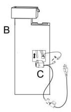
**Step 3:** Fill the basin (B) with clean water, making sure the pump (C) is fully submerged. **Note:** The maximum water level should be approximately 1.2 inches below the top edge of the basin (B).
