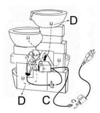
**Step 3:** Fill the basin (B) with clean water, making sure the pump (C) is fully submerged. **Note:** The maximum water level should be approximately 1.2 inches below the top edge of the basin (B).
