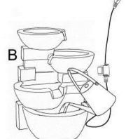
**Step 4:** Finally, connect the plug of pump (C) to a GFCI outlet.
