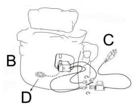
**Step 3:** Fill the basin (B) with clean water, making sure the pump (C) is fully submerged. **Note:** The maximum water level should be approximately 1.2 inches below the top edge of the basin (B).
