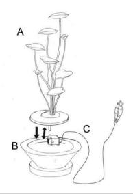
**Step 2:** Fill the basin (B) with clean water, make sure the pump (B) is fully submerged. **Note:** The maximum water level should be approximately 1.2 inches below the top edge of the basin (B).
