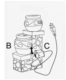
**Step 3:** Fill the basin (B) with clean water, making sure the pump (C) is fully submerged. **Note:** The maximum water level should be approximately 1.2 inches below the top edge of the basin (B).
