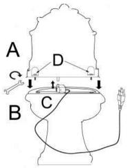
**Step 3:** Fill the basin (B) with clean water, making sure the pump (C) is fully submerged.
