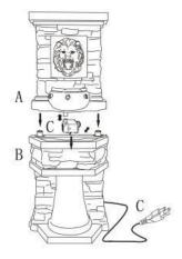
**Step 2:** Fill the basin of the bottom basin (B) with clean water, making sure the pump (C) is fully submerged.
