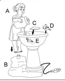
**Step 3:** Fill the basin (B) with clean water, making sure the pump (E) is fully submerged. **Note:** The maximum water level should be approximately 1.2 inches below the top edge of the basin (B).
