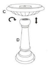
**Step 4:** Carefully attach the assembly from step 1 to the large basin (C), making sure to connect the water hose to the pump (F), and leave the pump in the bottom of the large basin (D).
