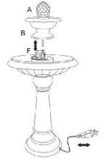
**Step 5:** Fill the basin (C) with clean water, making sure the pump (F) is fully submerged. **Note:** The maximum water level should be approximately 1.2 inches below the top edge of the basin (C).
