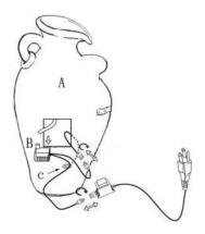
**Step 2:** Fill the basin of the polyresin pot (A) with clean water, making sure the pump (B) is fully submerged.
