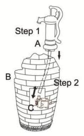
**Step 3:** Fill the basin (B) with clean water, making sure the pump (B) is fully submerged. **Note:** The maximum water level should be approximately 1.2 inches below the top edge of the basin (B).
